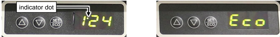
Figure 12. The Störk ST25-Eco controller. (Left) The lit indicator dot signifies that the heating element is activated. (Right) the controller in ECO-mode.
