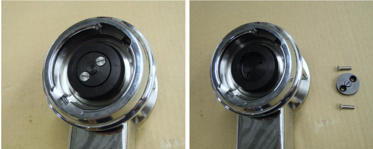
Figure 18a (left). Dispersion set (POM material) mounted in group head.
