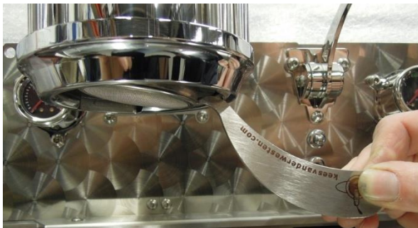
Figure 17 a (left). Pry left and right with screen extractor to remove group screen and group seal.
