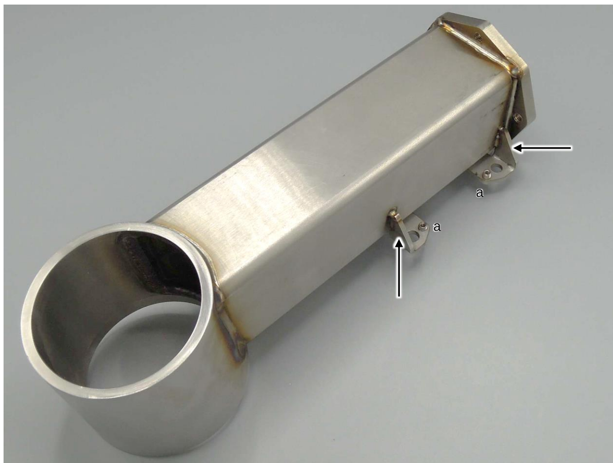
The photo above shows an untreated prototype of the bare boiler with reinforced mounting
