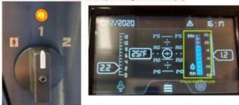
If machine has timed out, cycle machine off/on (position "1") again and allow to auto fill. If machine is still timing out, shut machine down and re-check the inlet water line / filtration system and confirm water flow to machine.
